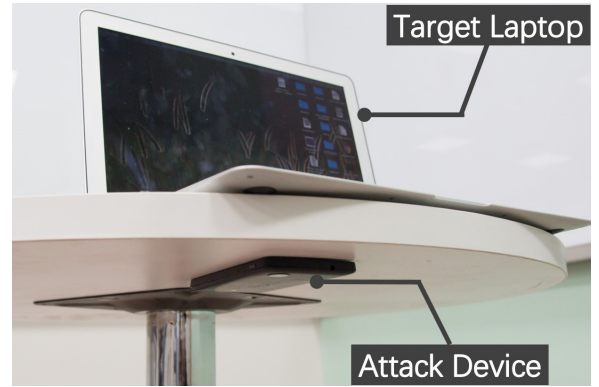
Figure 7: The experimental scenario of MagAttack. We keep the attack device under the table to draw no attention. The round table is 2.5 cm in thickness.
